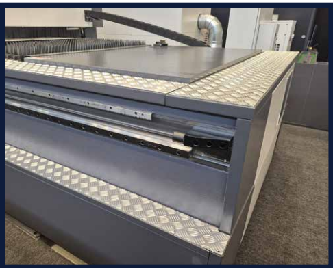
RACK AND PINION SYSTEM
