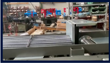
BUNDLE STOP TO BUNCH UP RE-BAR
