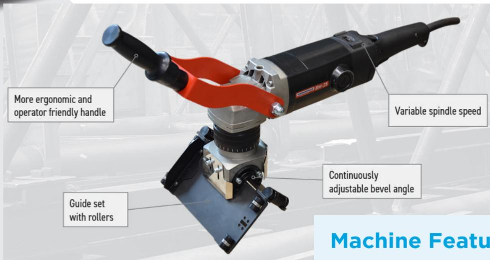
The BM-25 is an easy-to-use, portable, heavy-duty machine, enabling bevels up to 25 mm wide. The beveller is equipped with powerful motor and fitted with face milling beveling head, allowing smooth operation and exceptional efficiency. BM-25 enables milling straight edges up to 25 mm bevel width, whereas variable spindle speed facilitates optimizing cutting conditions. Continuously adjustable milling depth and bevel angle between 0 and 90 require no tooling to change.
