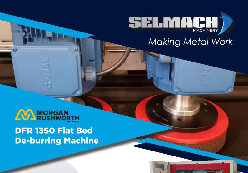
The Morgan Rushworth DFR 1350 Flat Bed De-burring Machine is a robust and cost-effective solution for de-slagging and deburring profile cut parts. The machine can process parts in the thickness range of 0 – 40mm and up to 1350mm wide. A conveyor with adjustable speed moves the parts through the machine while two pairs of oscillating wheels perform the de-burring action.
