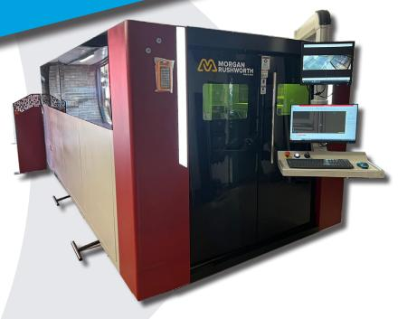
The Morgan Rushworth XL range of fibre laser cutting machines are equipped with a 3m x 1.5m or 4 x 2m cutting area with automatic shuttle table with dual pallet changer, enabling parts to be safely loaded and unloaded whilst the machine is still cutting. Class leading components ensure superior cut quality, high reliability and reduced down time.
