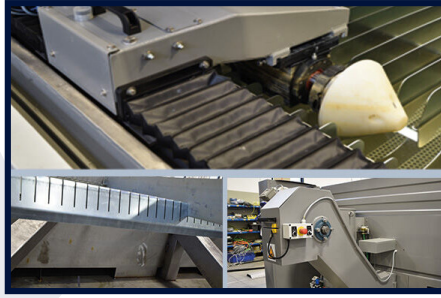
BELLOWS PROTECT LINEAR RAILS FROM DUST AND ABRASIVES
