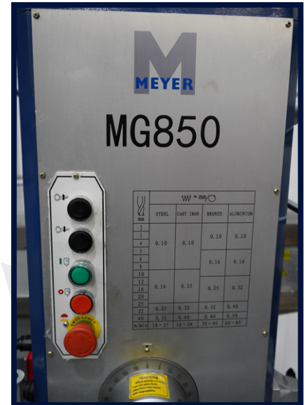
MG850 MAIN CONTROL PANEL
