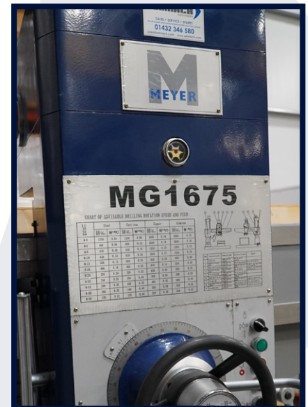
MG1675 MAIN CONTROL PANEL
