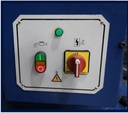
POWER CONTROL PANEL
