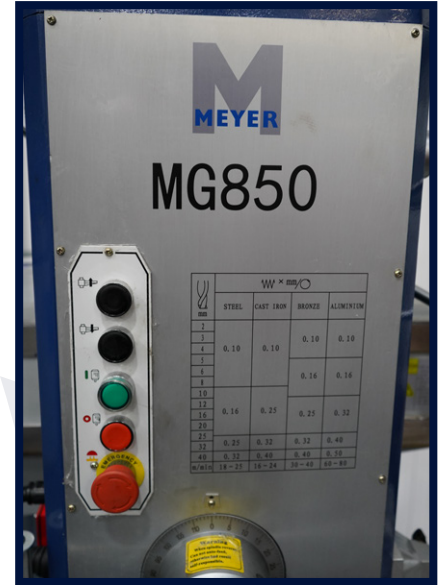
MG850 MAIN CONTROL PANEL
