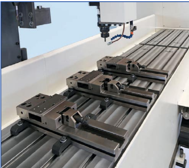
MULTIPLE SMALL PARTS CAN BE PRODUCED BY COPYING AND NESTING THE PARTS IN THE PROGRAMMER
