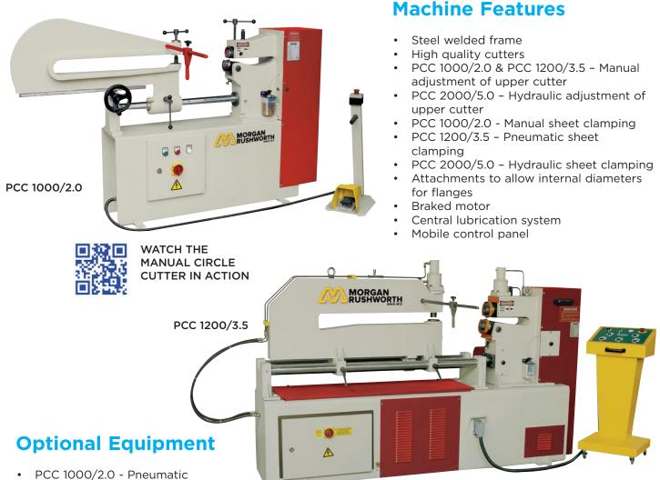
PCC 1000/2.0 - Pneumatic sheet clamping
