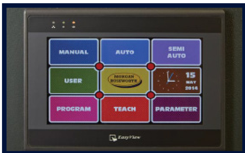
NC CONTROL PANEL SCREEN
