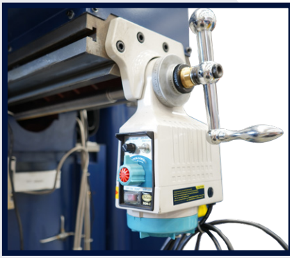
POWER FEED UNIT
